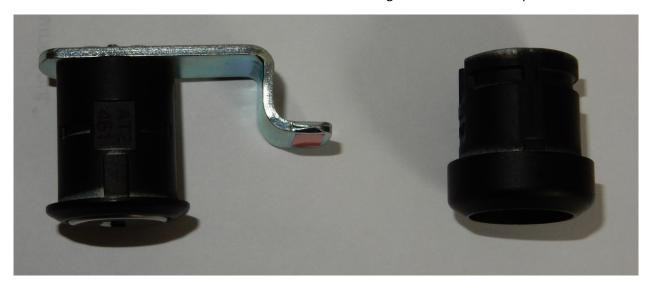
The original Tracer 700 lock is on the left hand side in the photo with the lock bar attached and the other lock casing is the one included in the kit. Other bikes lock casing may be used on other bikes; all that matters is that the lock barrel fits snugly in to the casing.
